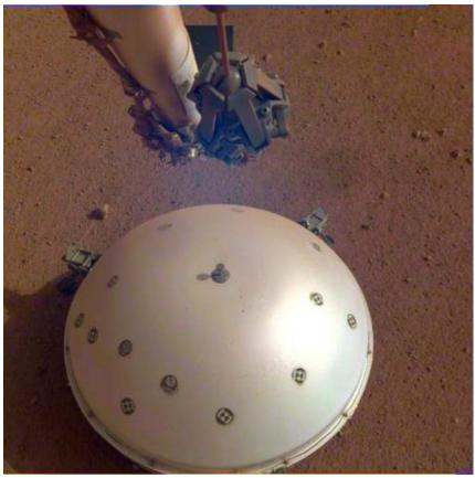
**InSight's Seismometer:** InSight's domed Wind and Thermal Shield covers the lander's seismometer, called Seismic Experiment for Interior Structure, or <u>SEIS</u>. The image was taken on the 110th Martian day, or sol, of the mission. Credit: NASA/JPL-Caltech. <u>Download image</u>
