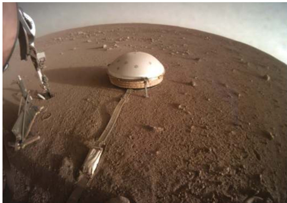
The Mars lander's seismometer contains three sensitive sensors nestled inside a dome.
